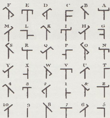
A key to the letter and number positions in the Chappe signaling system.
